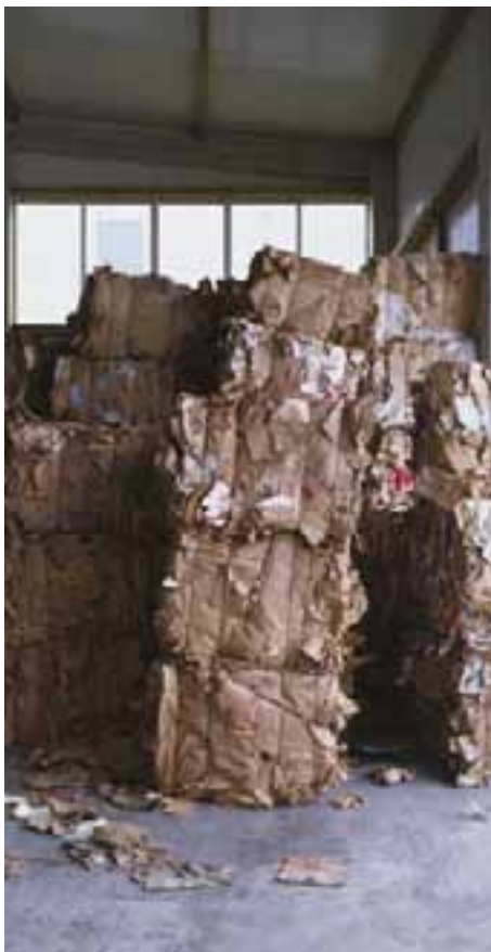
An important ingredient of our calcium sulphate panels are cellulose fibres which we obtain from recycled paper.
